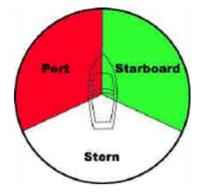
The port sidelight displays a red-coloured light through a horizontal arc (angle) of 112.5° from straight ahead to 22.5° abaft the beam. The starboard sidelight displays a green-coloured light through a horizontal arc (angle) of 112.5° from straight ahead to 22.5° abaft the beam. The stern light is whitecoloured, shines directly aft, and displays light through a horizontal arc (angle) of 135° across the stern.
